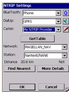
7. To choose a station from which to receive RTCM corrections:
