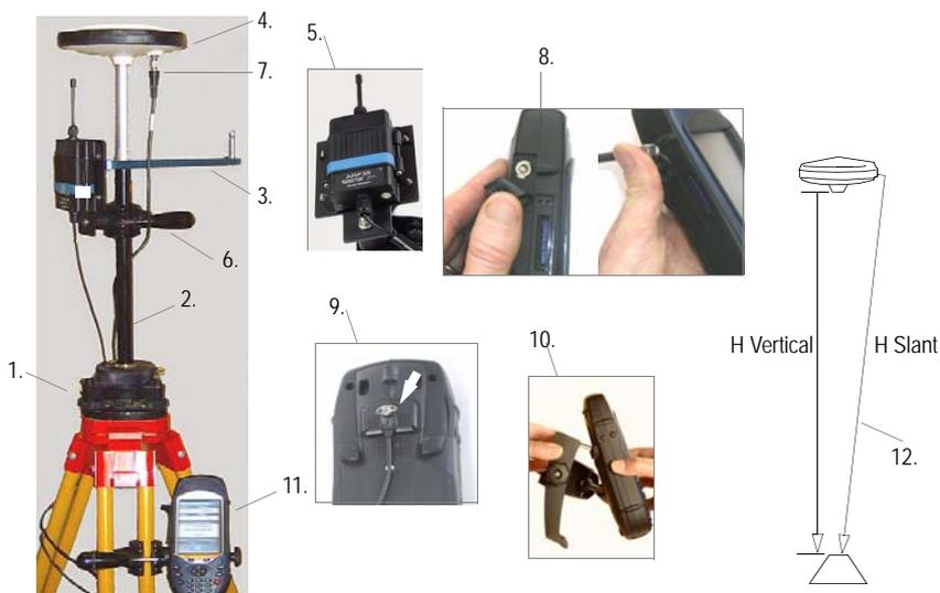
1. Set up the tripod / tribrach combination over the point.
