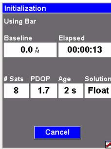
6. Keep an eye on the displayed parameters while the receiver initializes:
